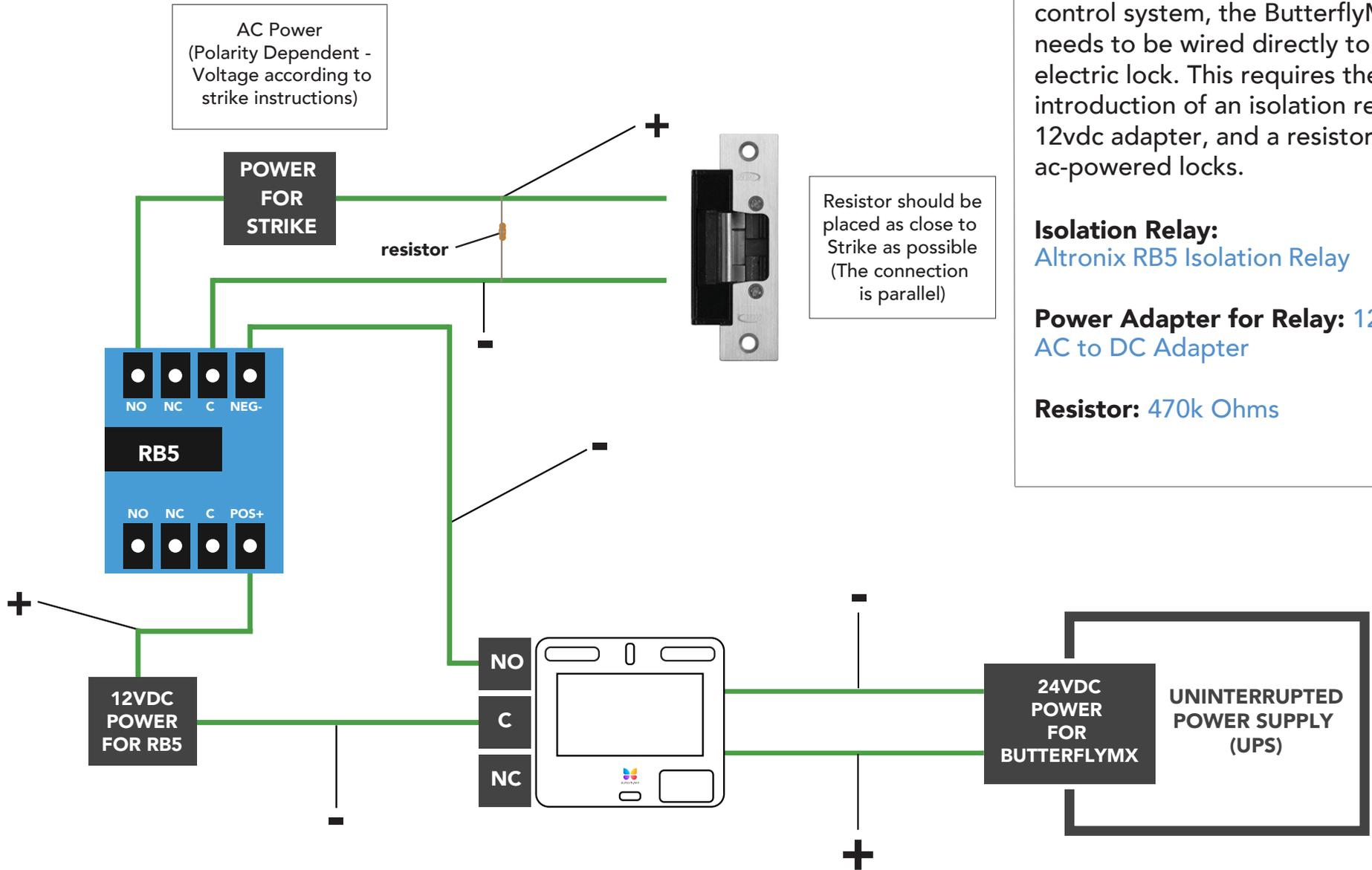
When installing a ButterflyMX panel at a building without an access control system, the ButterflyMX needs to be wired directly to an electric lock. This requires the introduction of an isolation relay and 12vdc adapter, and a resistor for ac-powered locks.
